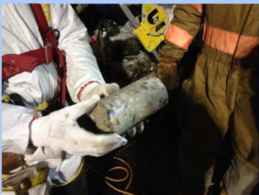
Cores taken for structural analysis, 6-7 February 2014
