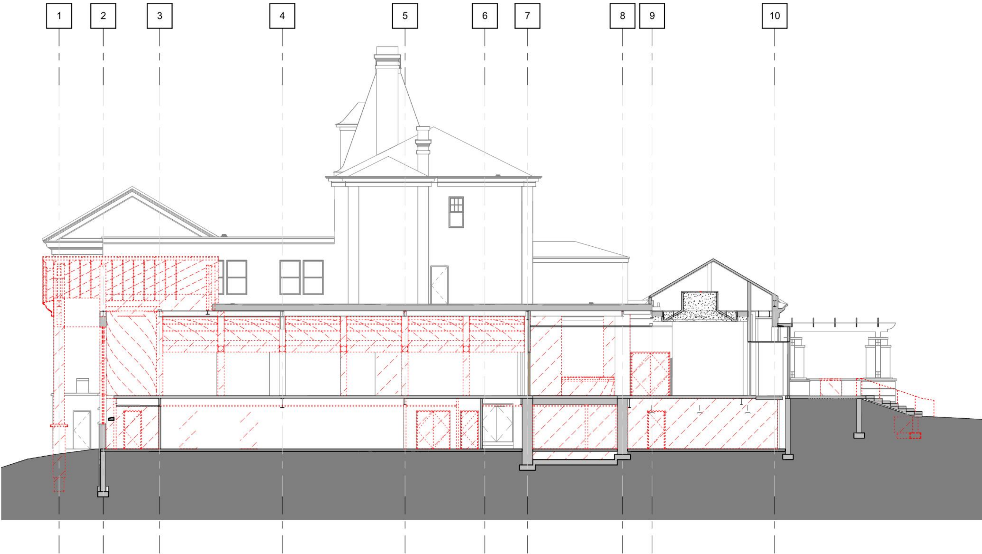
CROSS SECTION - DEMOLITION AT EX. ENTRY 1.22 | 1.26 3/32" = 1'-0"
